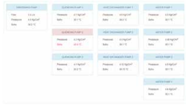
Application Example: Custom Dashboard view to monitor pressure, temperature and flow of water pumps
